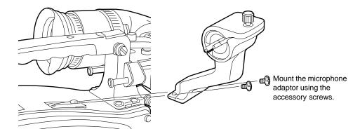
3 Mount the microphone to the microphone holder and tighten the screws.
